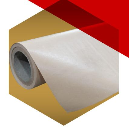
This calendered Kraft-style **release paper** features a specialized silicone non-stick coating on both sides. It's designed for use between uncured rubber and the vulcanizing press during belt splicing. Ideal for step, finger, and steel cord splicing, it works across all belt types and
