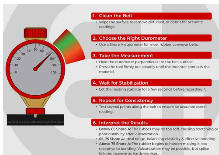
Figure 2. A durometer measures belt hardness in Shore A units.
