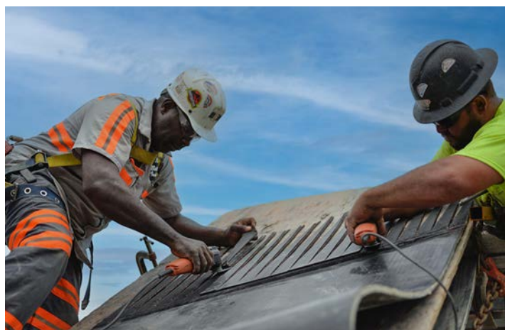
Figure 3. A crew expertly splicing a conveyor belt, a process requiring precision to ensure long-term durability and performance.
